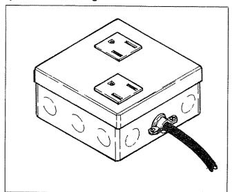
One method of connecting a 3-wire cable is to terminate the cable at an outlet box, as shown above
